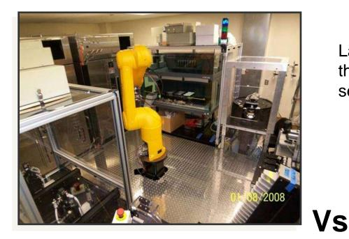
Large motion-controlled systems that perform multiple tasks by integrating several robotic devices.
